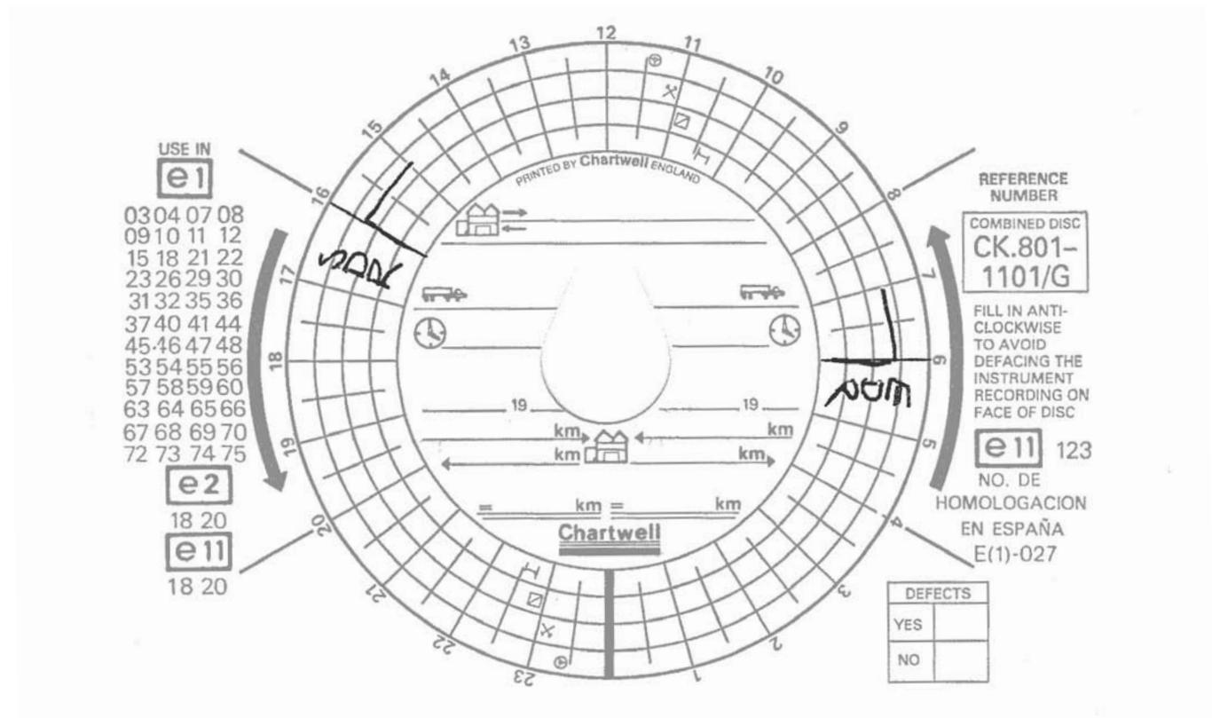
This is an example of manual entries made on the rear of a tachograph chart by a driver who started his day at 06.00 with an hour's work doing other duties away from his vehicle. He also finished his day with an hour of other work away from his vehicle and has indicated both the end and the start of a daily rest period. His activities while with the vehicle are recorded by the instrument on the other side of the chart once it has been inserted.
